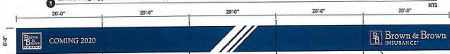
1 Elevation of Digitally printed Fence Scrim, Section (I) - reference below for widths each section will be fabricated, each section to have 3" bleed all sides
