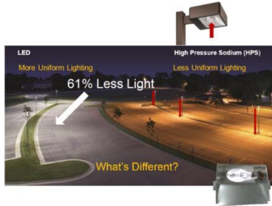
Comparison of LED fixtures (left) versus High Pressure Sodium (HPS) fixtures (right)
