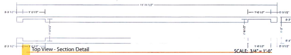
H S/F Brakeformed Alum. Gas Pump Canopy Spanner Panel (6.06 SQ FT) - QTY: 2 6.06' SF SCALE: 3/4" = 1'-0"
